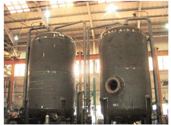
Pressure Vessels in Process
